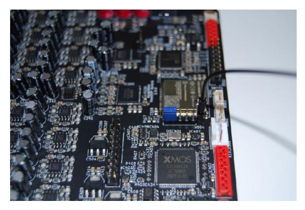
6. Connect TXD of your USB2Serial module with pin 4 of X504.
