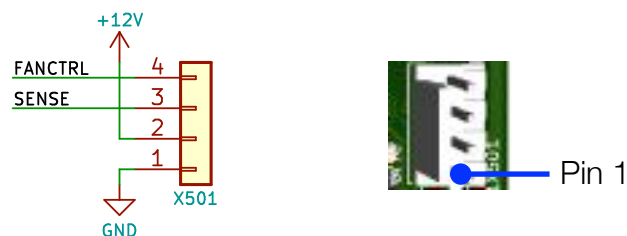
Pinout Fan and Temperature Sensor
